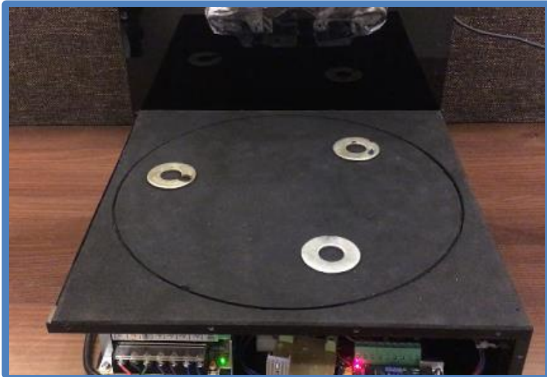
Lab Setup Emulating Conveyor Belt
